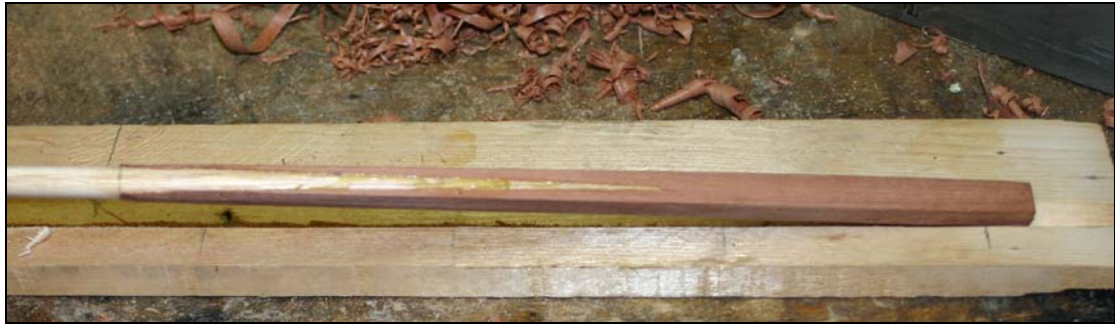
Figure 10 The wings have been planed down.
