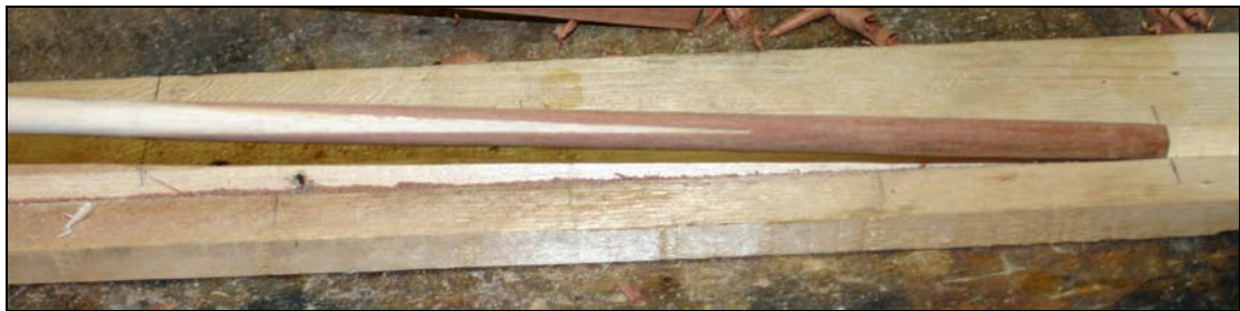
Figure 11 More planing to make it 16 sided and then sanded.
