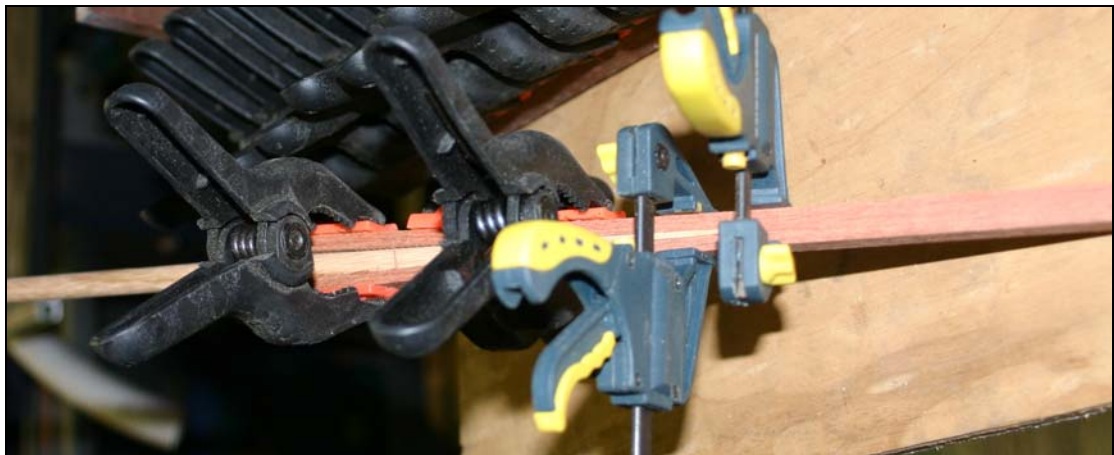
Figure 7 Shaft has been smeared with glue and inserted into foot and tapped home. Clamps have been applied to ensure good contact and resulting bond.
