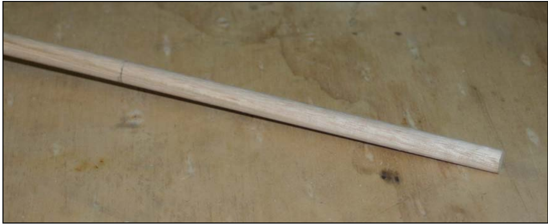
Figure 1 A blank shaft with mark for taper to be cut.
