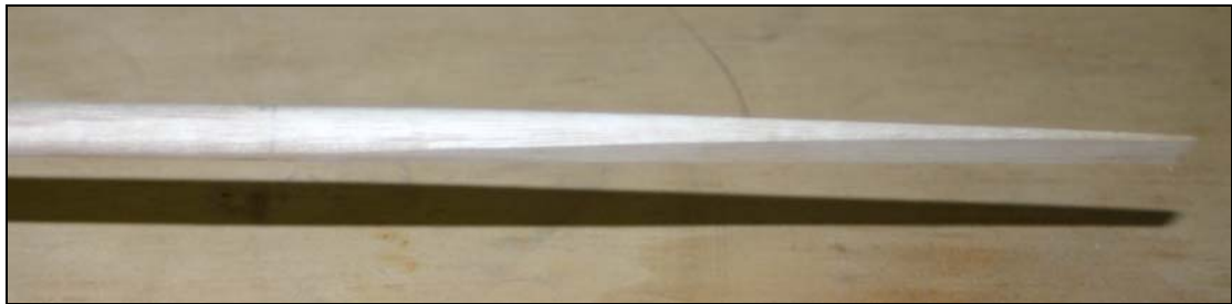
Figure 2 The end of the shaft tapered. Edge on view.
