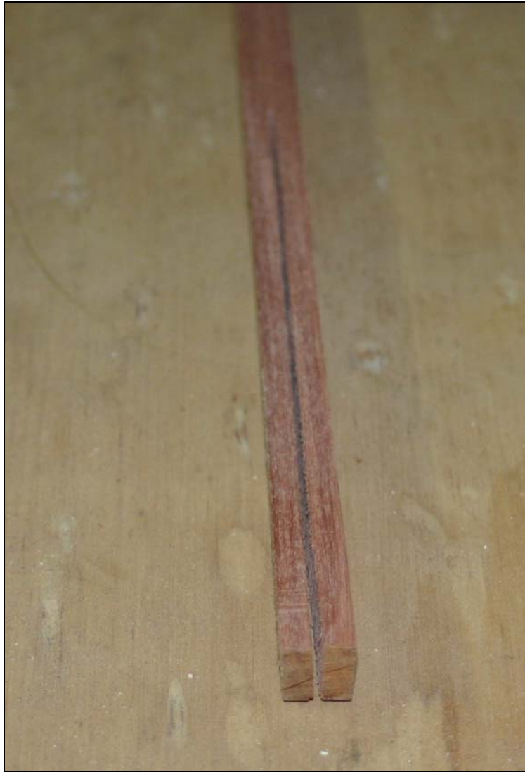
Figure 5 Foot has been split the required distance.
